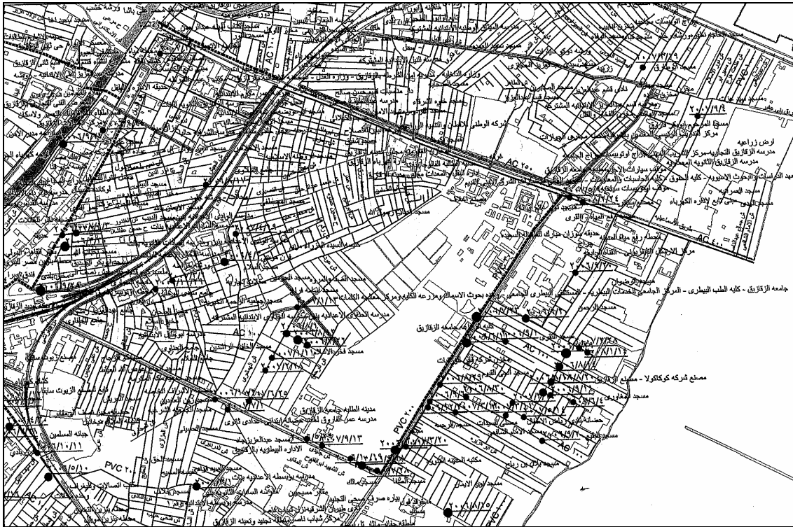
Figure 4.1-20 Location of Broken Pipes in Zagazig City-East
