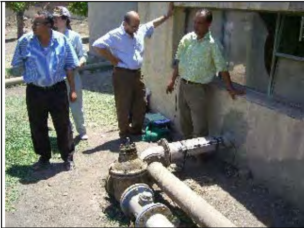
Measurement for well production by portable flow meter in Diarb Nigm Markaz. (Action S10) (Date: Jun.24, 2007)
