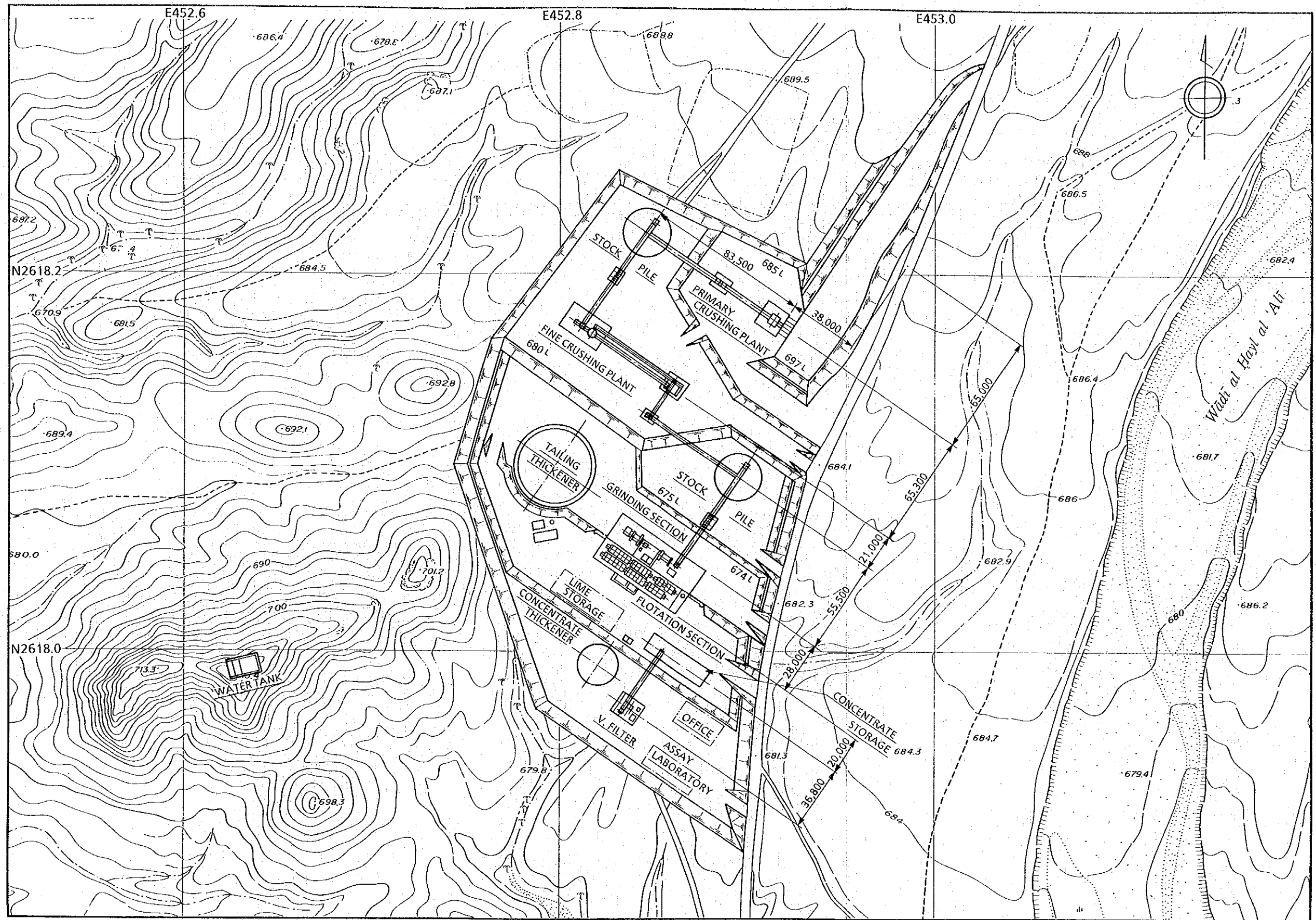
Fig. 1 General layout of mineral processing plant
