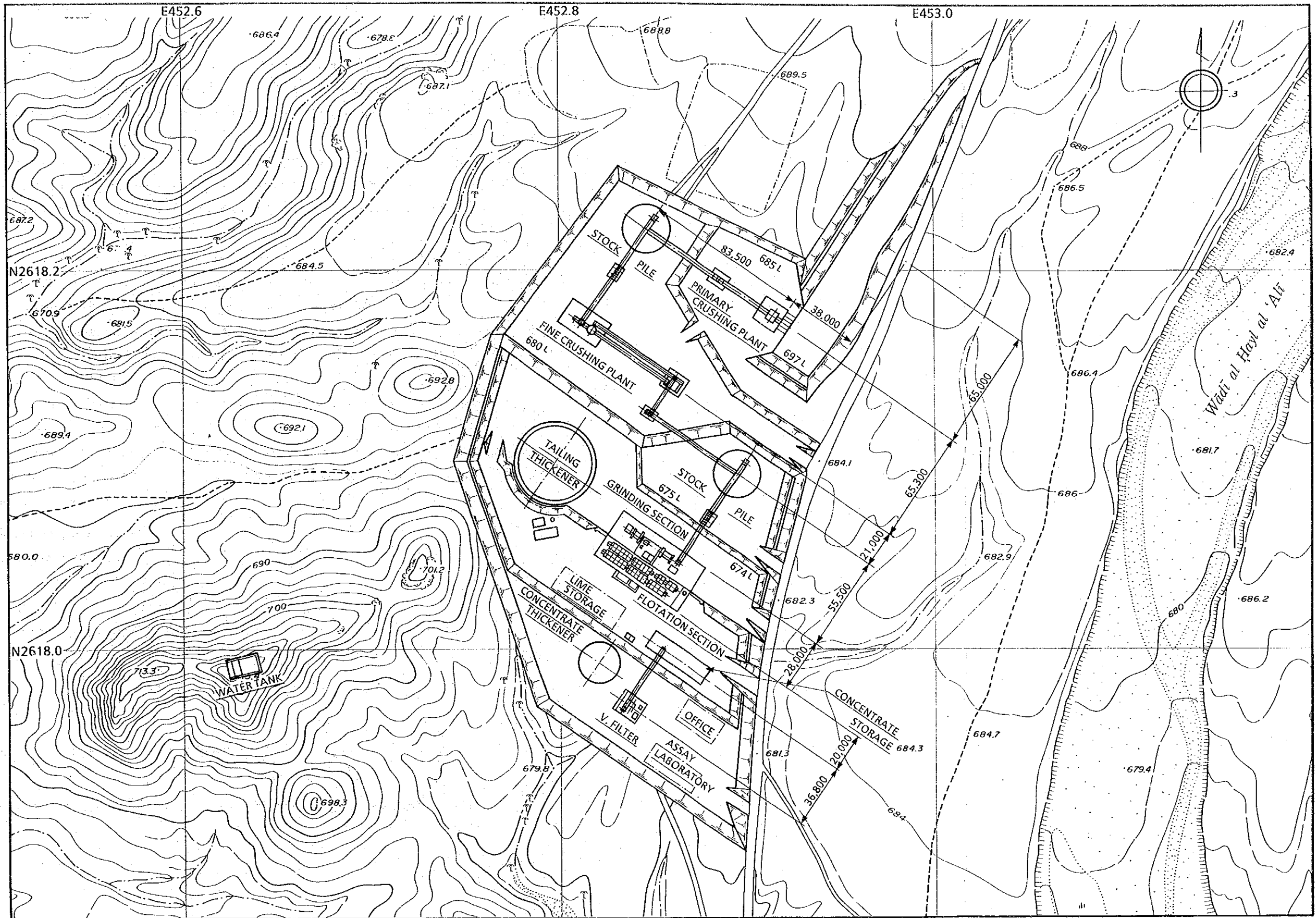
Fig. 9 General layout of mineral processing plant
