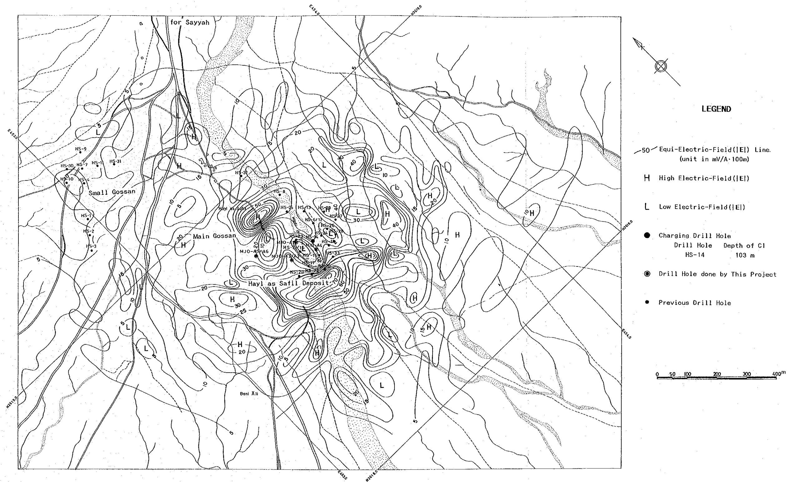
Fig. 1-22 Electric field map for the drill hole HS-14 in Area A
