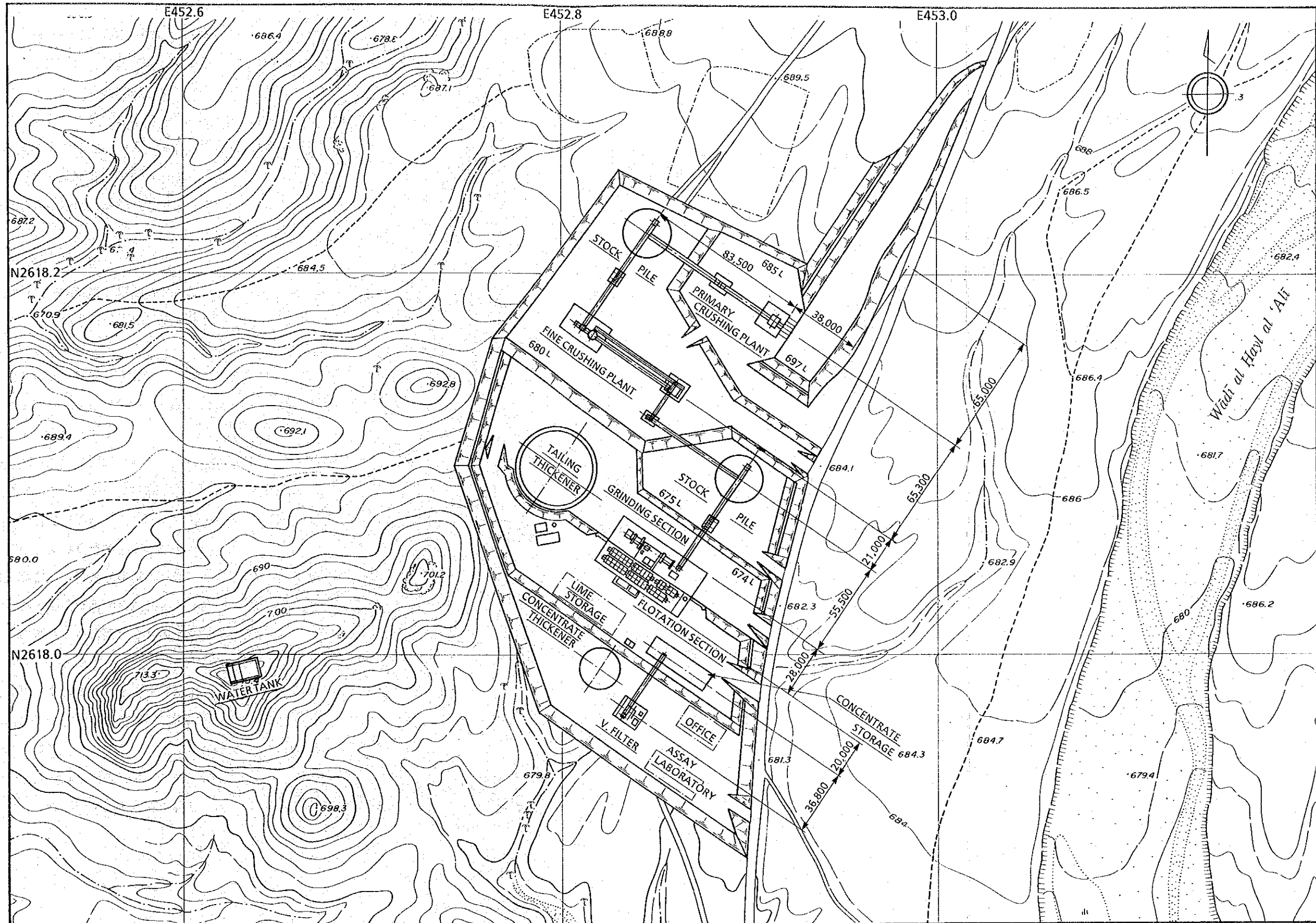
Fig. 9 General layout of mineral processing plant
