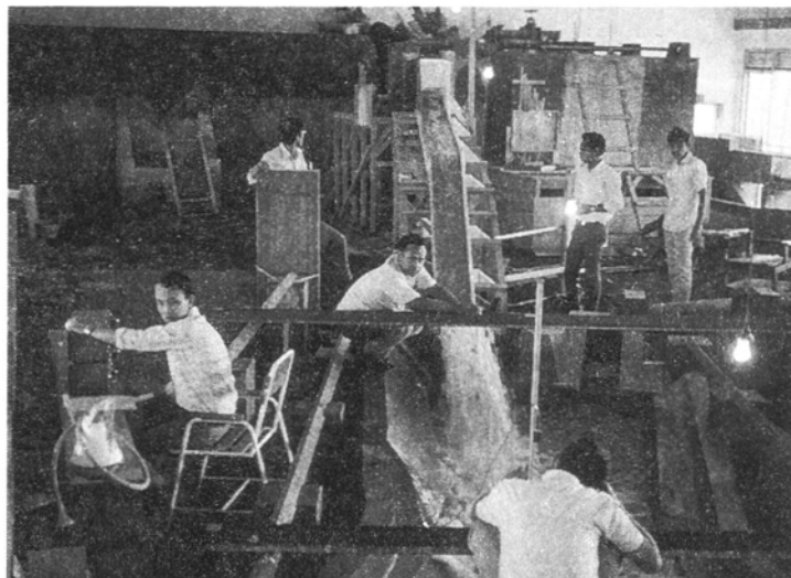
Hydraulic model experiment at Brawijaya University
