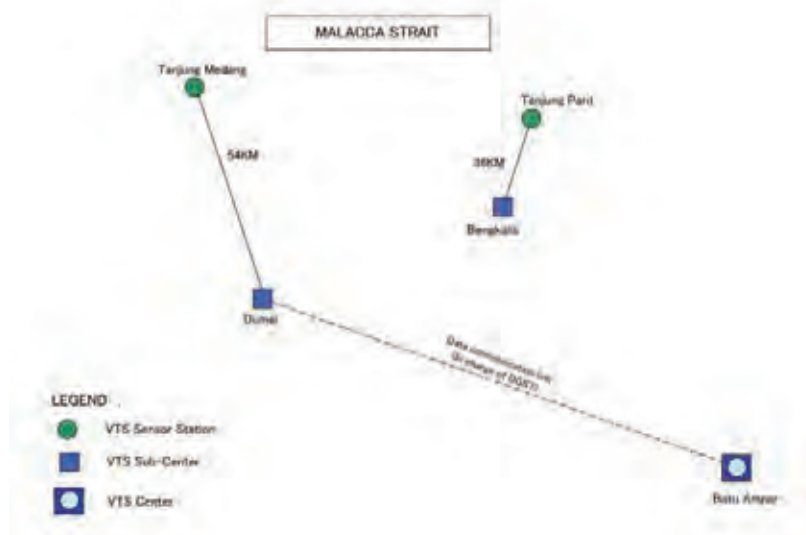
Fig. 2-1-2 VTS System Concept (by the BD Study)
