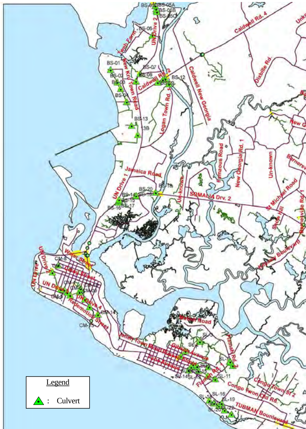
Figure 7.2-2 (1) Location of Culverts in the Priority Area
