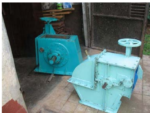
Turbines made in Switzerland (Left) and Uganda (Right)
