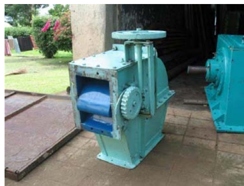
Cross Flow Turbine (28 W)
