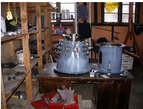
Turbine for Discharge of 1.2 m 3 /s, Head of 11 to 22 m and 100 kW
