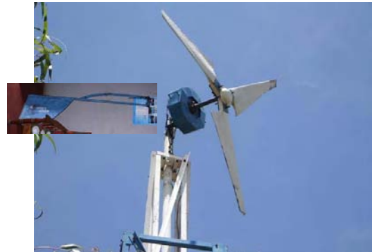
Wind Power Turbine (2.5 kW, Tail is broken.)
