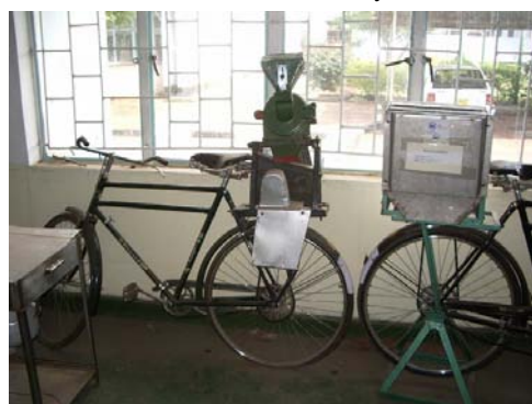
Flour Mill and Potato Slicer by Bicycle Power
