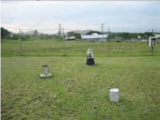
Meteorological observation station in Port Moresby in Papua new guinea. Due to Lack of instruments and old instruments, basic data cannot be obtained.
