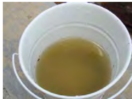
Figure 2.1.16 Effluent of Septic Tank
