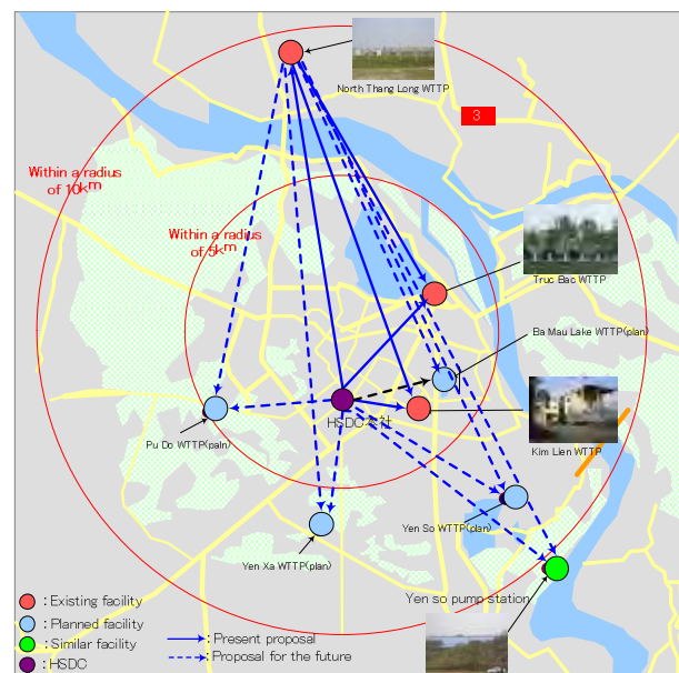
Integrated WWTP Monitoring System for Hanoi
