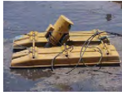
Figure 2.1.42 Surface Aerator with Inclined Screw Shaft
