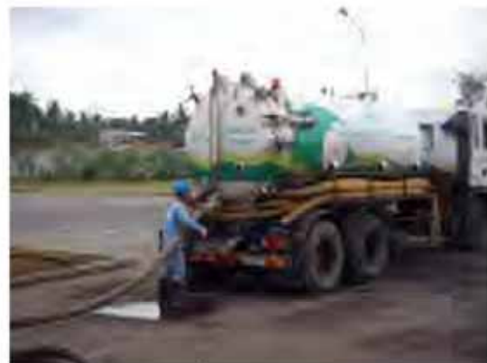
Photo 2.3.8: A 10 m 3 vacuum truck unloading septage at the MWCI San Mateo (South) septage treatment plant
