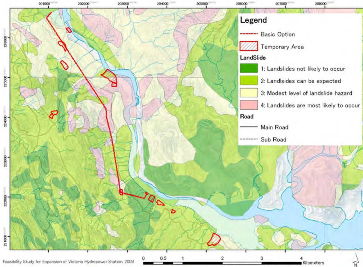
Figure 3-13 Landslide Zonation map
