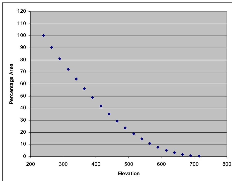
**Figure 3-2 Area Altitude Curve of the Project Impact Area (Basic Option)**
