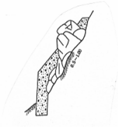
(Concrete foot protection work)
