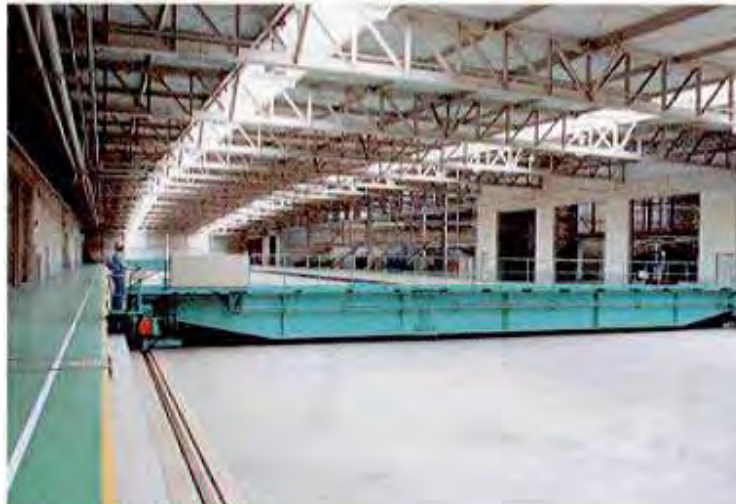
Photograph 32.1 Example of traverser table (in a factory)
