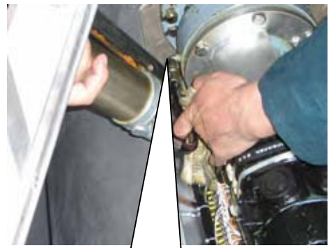
Inject grease through the grease nipple
