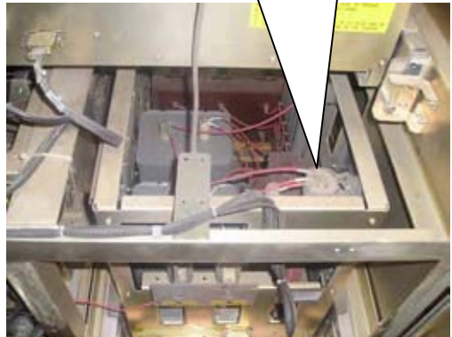
HV PS-1 Remove dust from high voltage parts
