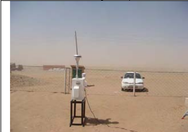
DSS Monitoring System Comparison sampling of PM10 Zamin-uud Observatory
