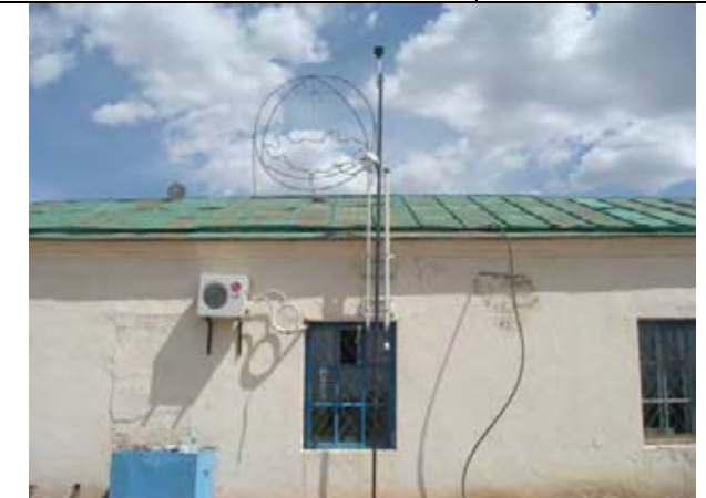
DSS Monitoring System Adjustment of the sampler's inlet Dalanzadgad aimag center
