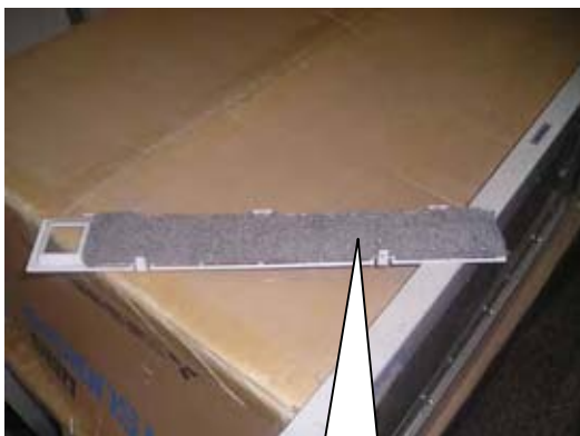
Air Filter Before cleaning
