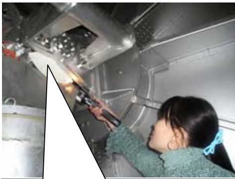
Checking of the Antenna elevation positioning accuracy (Reading the pointing angle on the mechanical scale of elevation angle)
