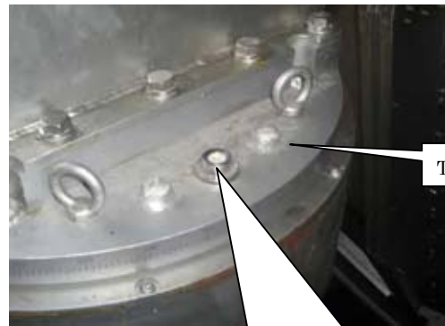
Check the level of the turn table on every 60 degree in Azimuth angle by this level
