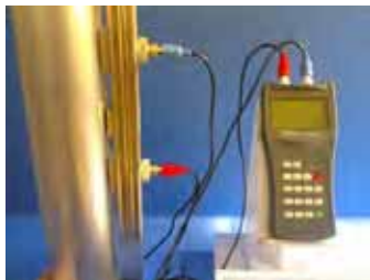
Potable Flow Meter (Ultra Sonic Flow Meter)
