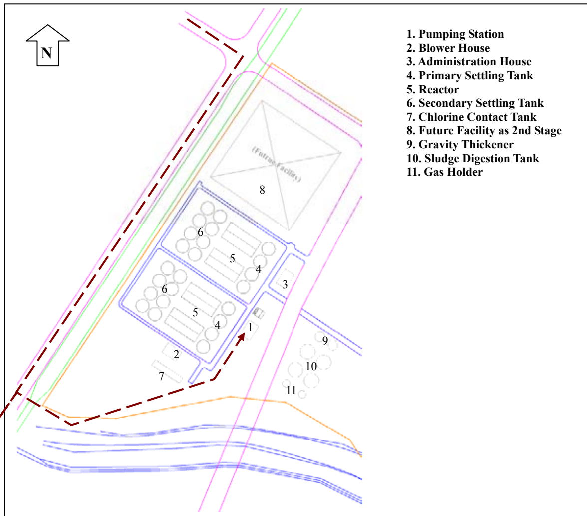
Figure 3.3 Layout of Treatment Facilities (1)
