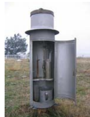
Normal Rain Gauge Used in Skopje City
