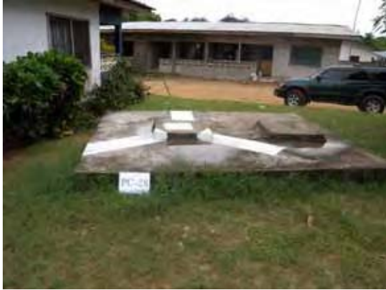
*Left Photograph shows a sample of pre-marked Control point.
