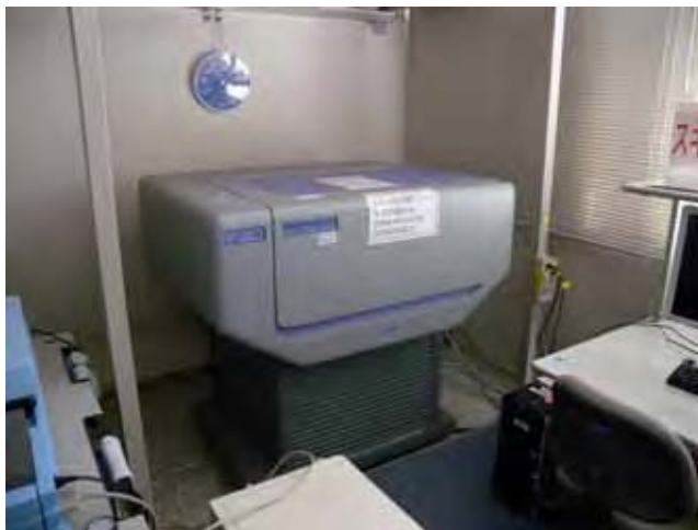
*Left photograph shows LEICA LH System, Photogrammetric Scanner, DSW500 (Digital Scanning Work Station Type 500)
