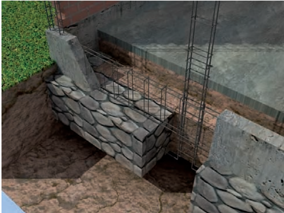
Picture of the constructive process of the foundation and the tie beam
