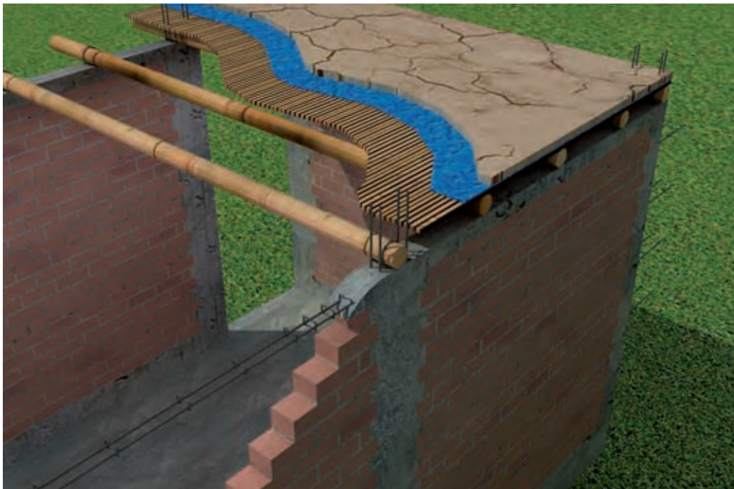
Picture of the constructive process of the cane roof
