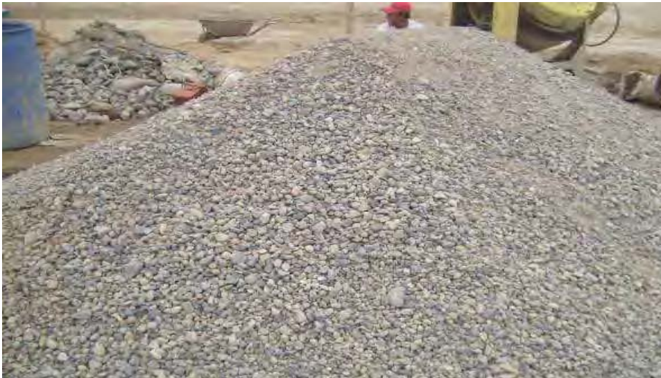
Clean crushed stone
