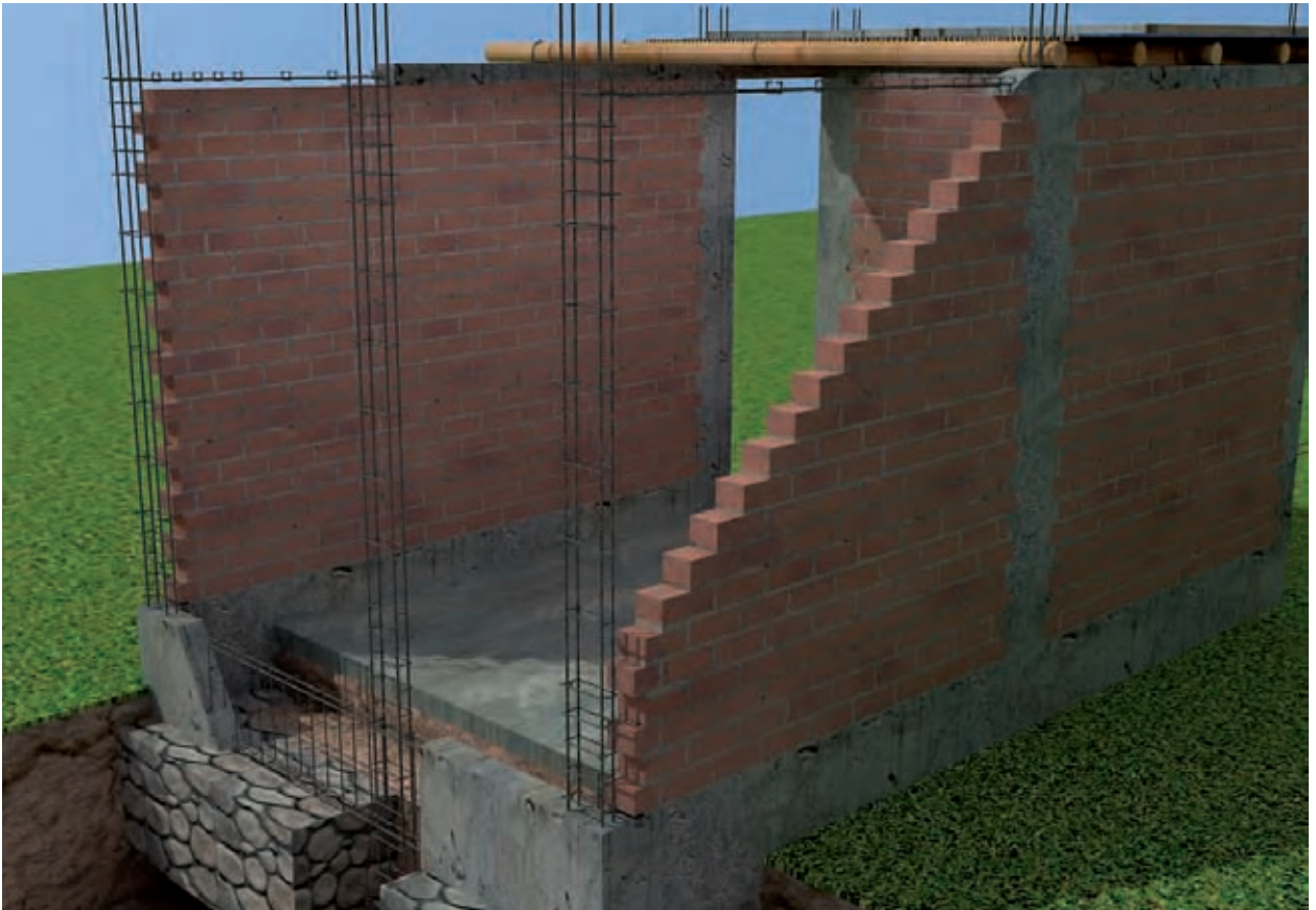
Picture of the constructive process of safer housing
