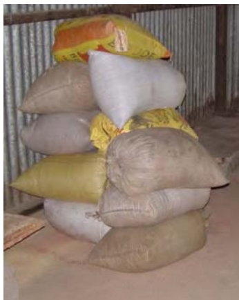
Photo 3.2-9 Example of Storage: Sacks Stored Directly on the Floor
