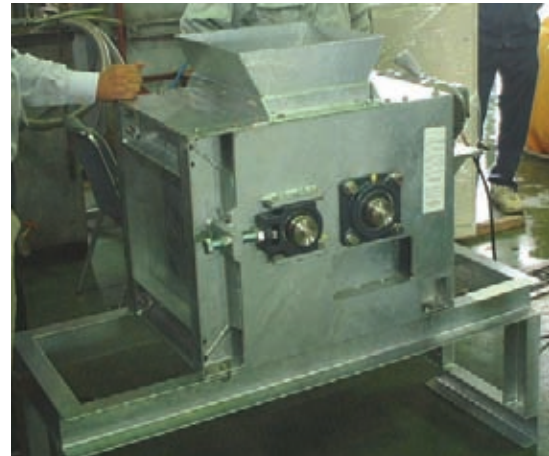
Fig. 2-21 Diagram and photograph of second-stage ice crusher
