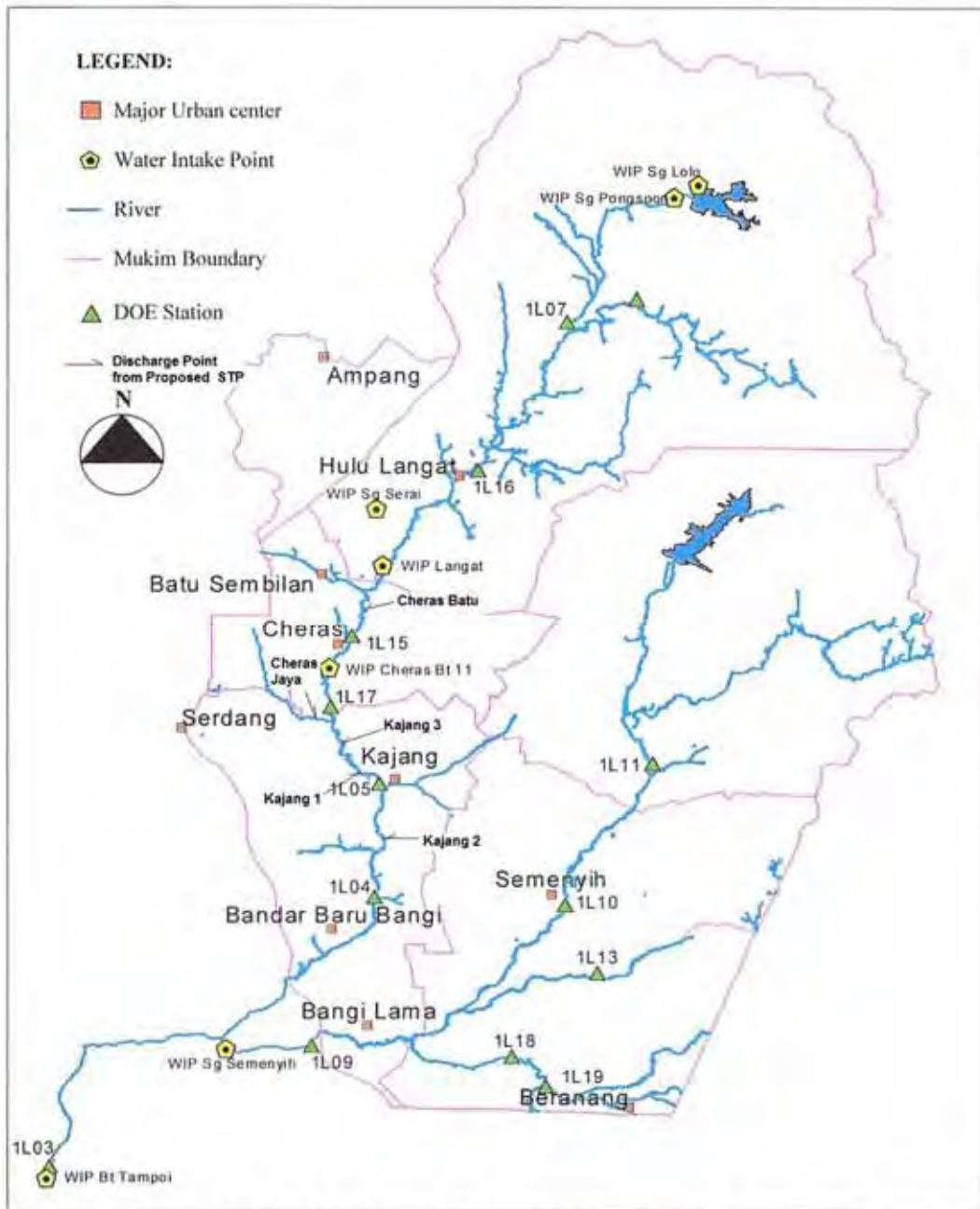
Figure 3.5.1 Location of DOE Monitoring Stations and Water Intakes in the Upper Langat River Basin
