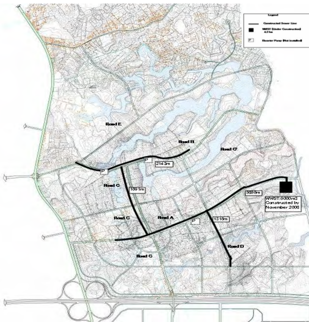
Figure E.1.1 Present Condition for Sewerage System
