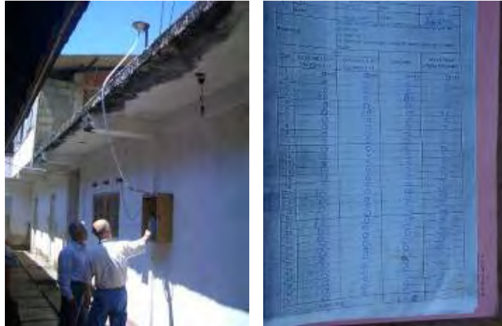
Figure M.3.16 Installed Rain Gauge Equipment and Rainfall Records by Residents
