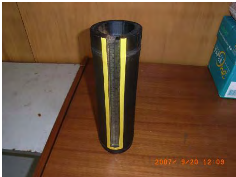
Figure 6.2.16 Handmade rainfall gauge made of bamboo
