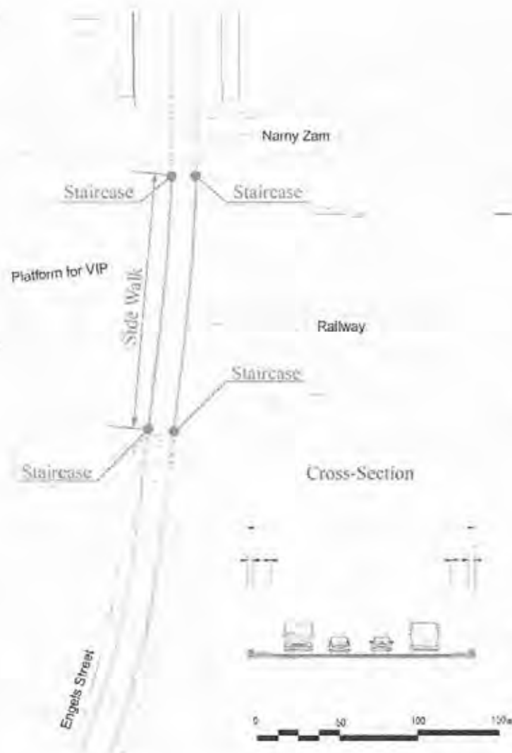
Fig. 2 Extent of Sidewalk on Railway Flyover
