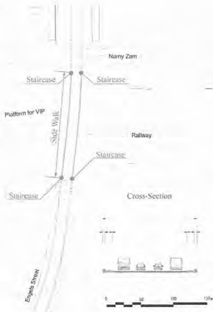
Fig. 2 Extent of Sidewalk on Railway Flyover
