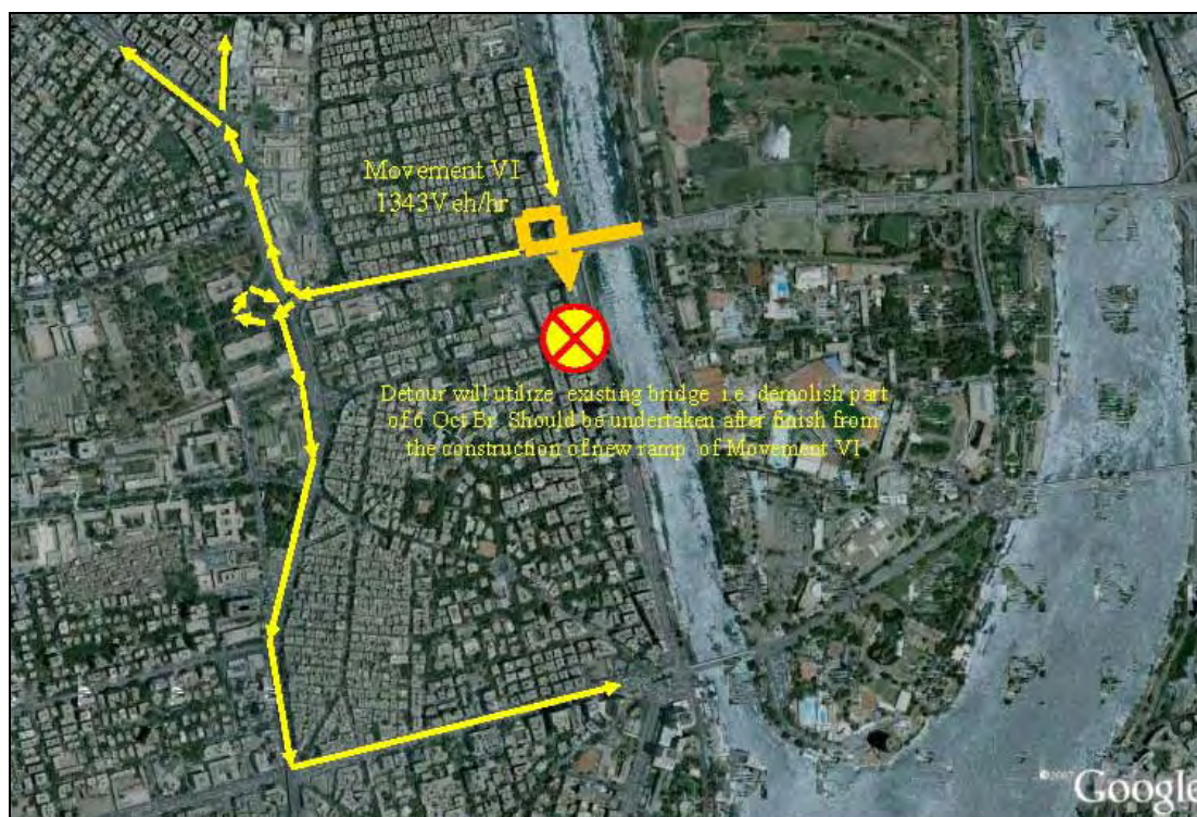
Figure 14.2-8 Detour of Traffic Movement VI
