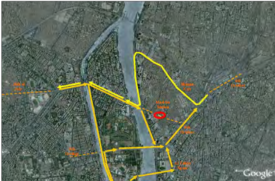
Figure 14.2-15 Detour Plan during Construction of Maspero Station
