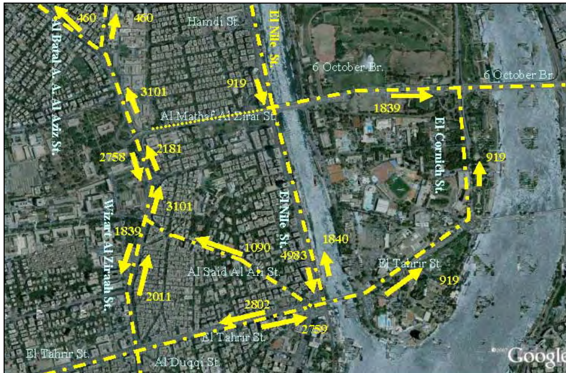
Figure 14.2-9 Assigned Detoured Traffic Movements 1, 2, 3 and 4
