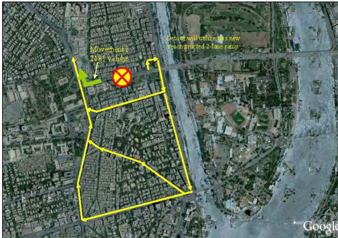
Figure 14.2-3 Detour of Traffic Movement I
