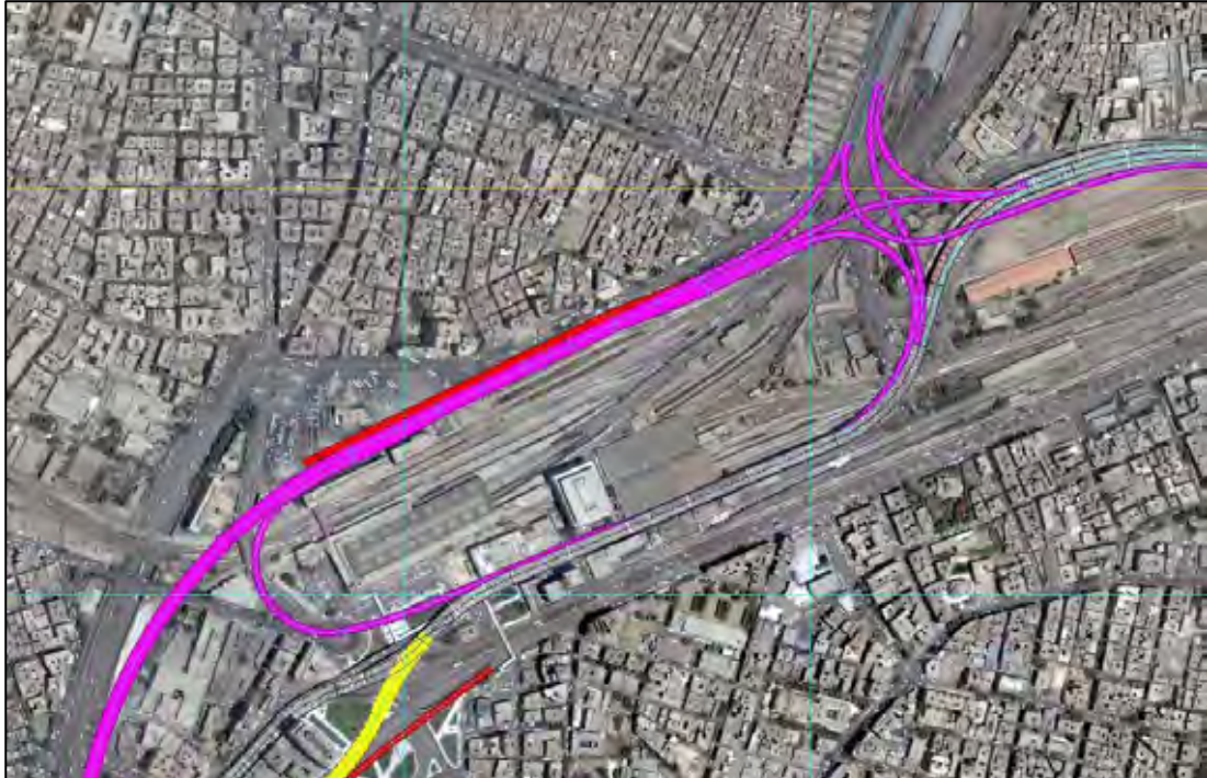
Figure 6.5-2 a Conceptual Layout Plan for E1-1 Bypass Extension with E5 Jct. (1) (Extension above Urabi St. Case)
