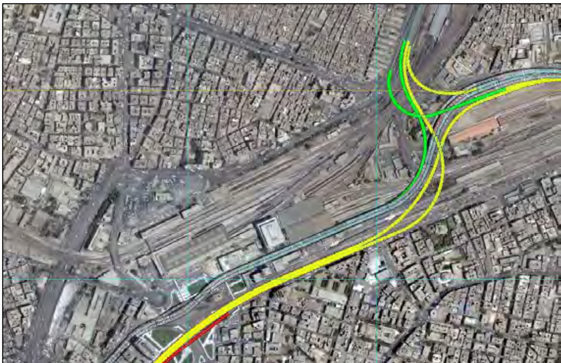
Figure 6.5-2 b Conceptual Layout Plan for E1-1 Bypass Extension with E5 Jct. (2) (Extension above Ramsis St. Case)
