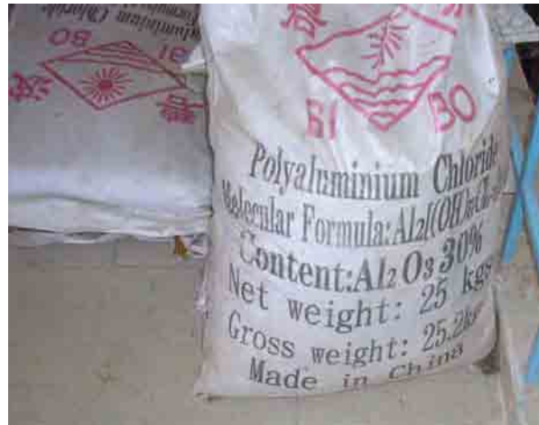
PAC as 30% Al 2 O 3 Xuan Phong water treatment plant in Khanh Hoa
