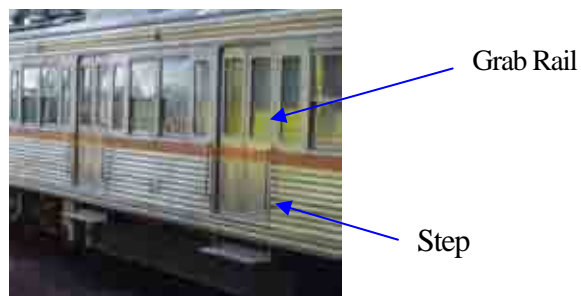
Figure 3 Steps and Grab Rail for Loading
