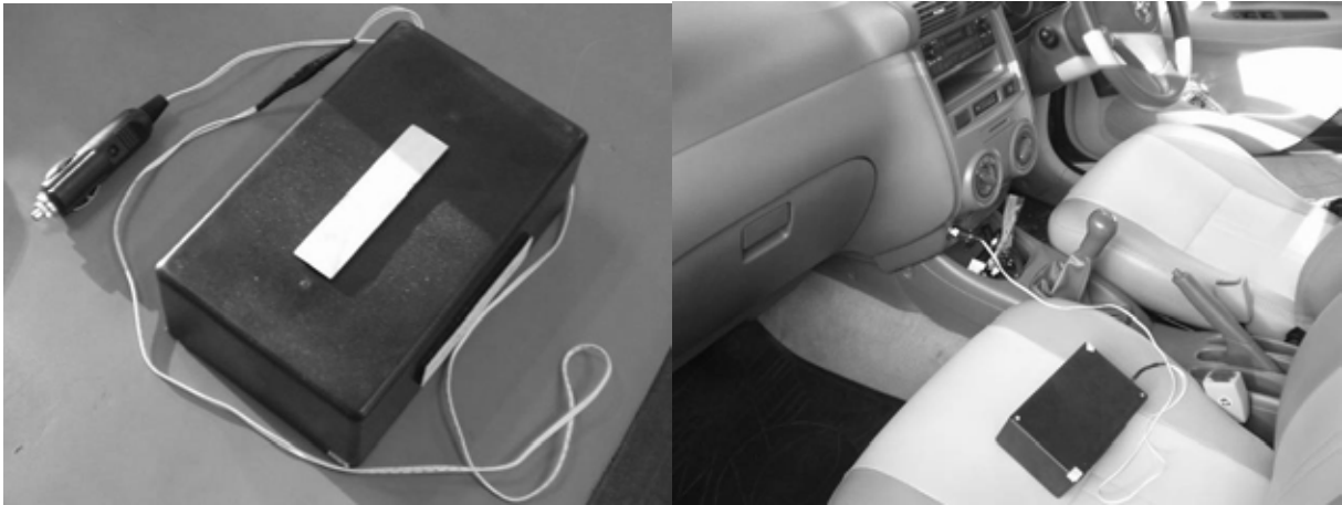
Figure 1.3.2 GPS device for Travel Speed Survey
