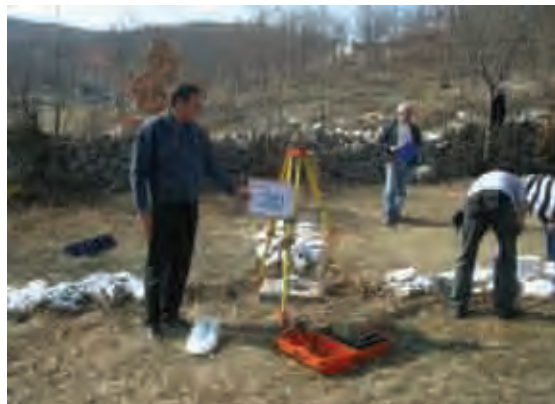
Photo 4 : Photo control point survey and air marking
