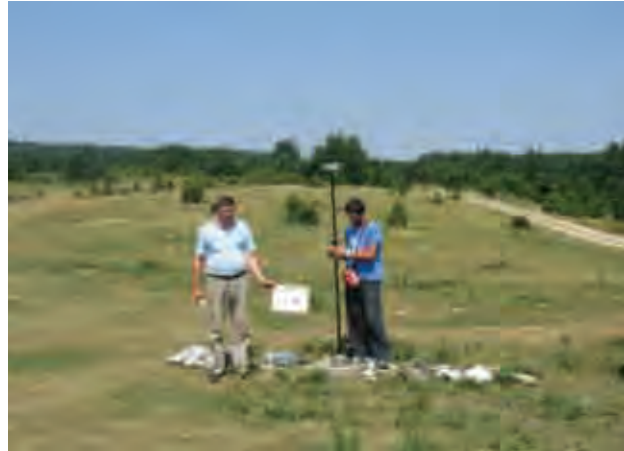
Photo 14 : GPS-based reference station on the roof of Pljevlja city office Photo 15 : Inspection survey of existing control point using RTK GPS
