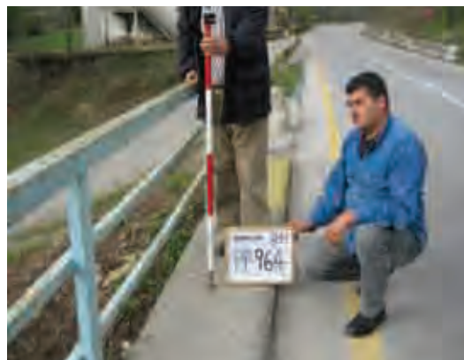
Photo 2 : Inspection survey using benchmarks
