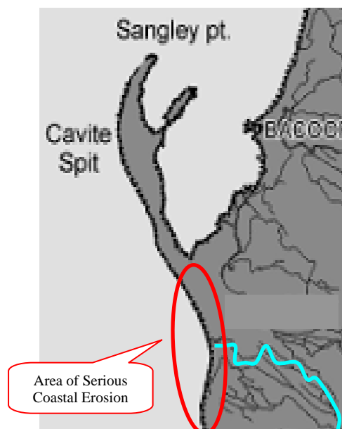
Fig. R 2.4 Erosion along West Shoreline of Cavite Spit
