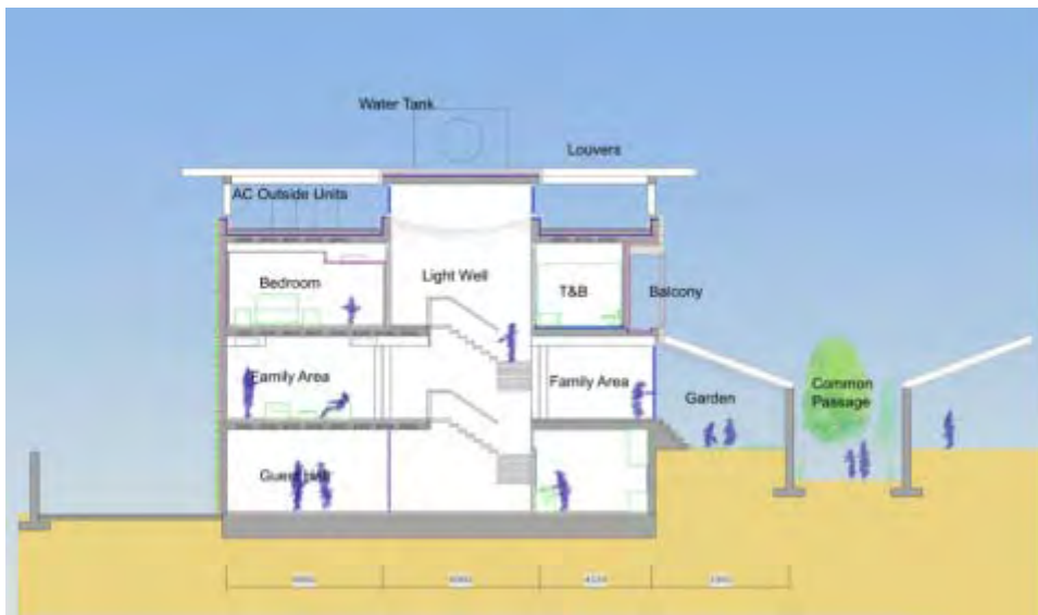
Figure AP4.1-23 Model House Section
