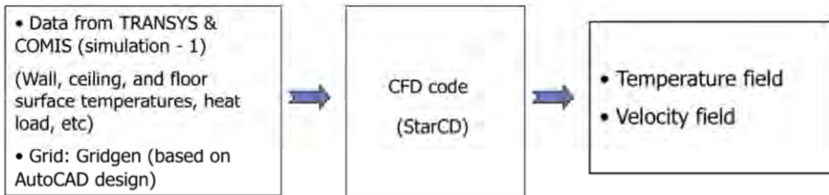
Figure AP4-1.50 Calculation Flow of CFD Simulation
