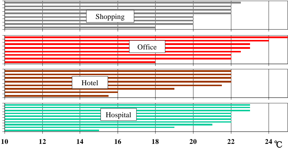
Figure AP1-66 AC Cooling Temperature
