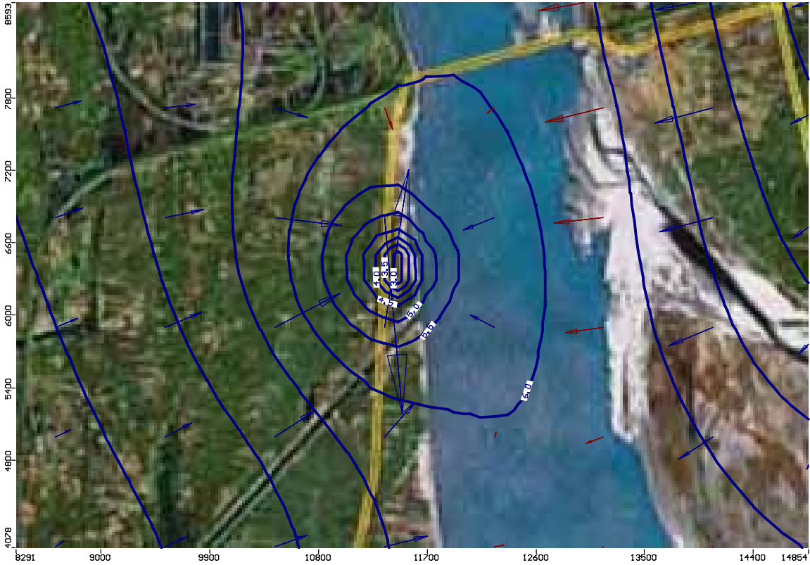
Figure 40. Zoomed in modelled dry season (May) water table contour map after 20 years of pumping (wells arranged in cluster).
