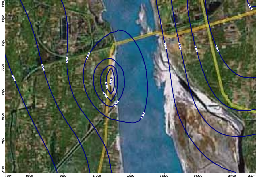
Figure 34. Zoomed in modelled dry season (May) water table contour map after 20 years of pumping (wells arranged in line).
