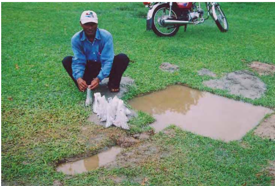
Photograph of SPT Sample of Bore Hole – 07 in field
