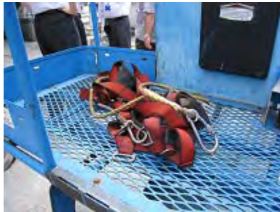
Thoroughly instructed to wear safety equipment (safety band for high-place work)
