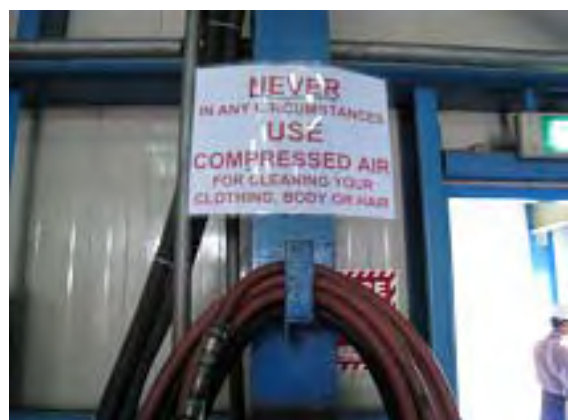
Safety sign (The use of compressed air to the body is strictly prohibited)
