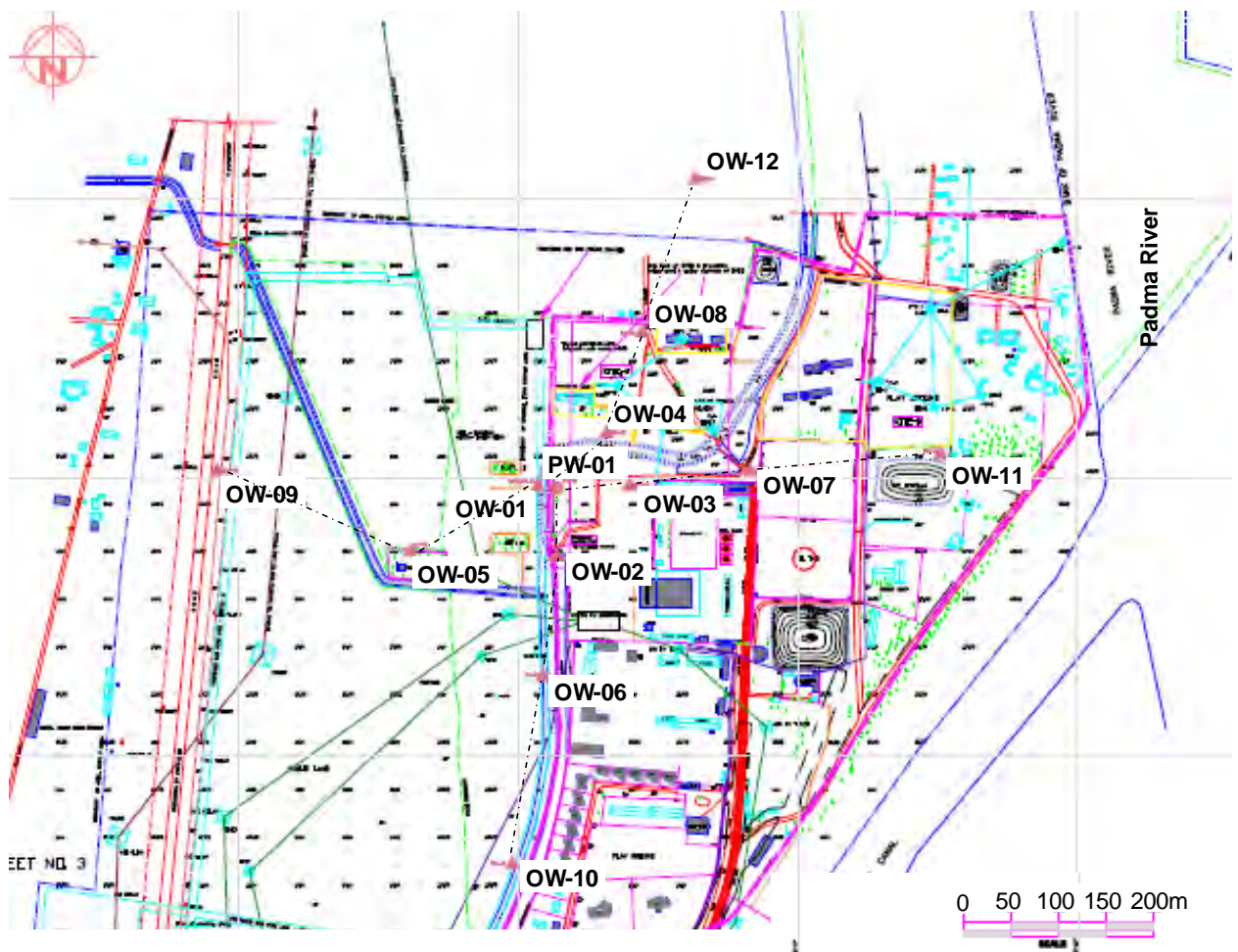
Figure I-4-6-10 Pump/Observation wells layout
