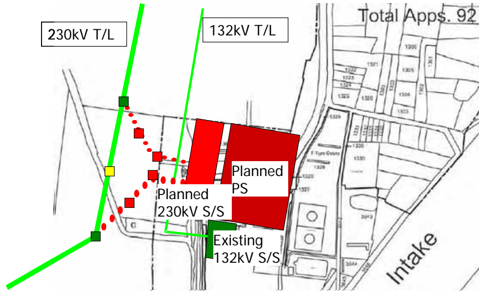
Figure I-4-4-2 Overview of transmission system around Bheramara substation
