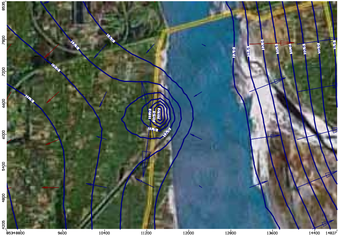
Figure 43. Zoomed in modelled wet season (September) water table contour map after 20 years of pumping (wells arranged in cluster).
