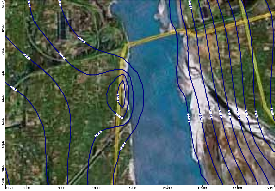
Figure 37. Zoomed in modelled wet season (September) water table contour map after 20 years of pumping (wells arranged in line).
