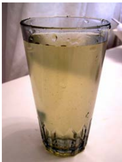
Supplied water coloured by iron
