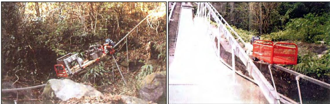
Figure 8.3.3 Examples of Simple Monorail Car Used on Steep Slopes
