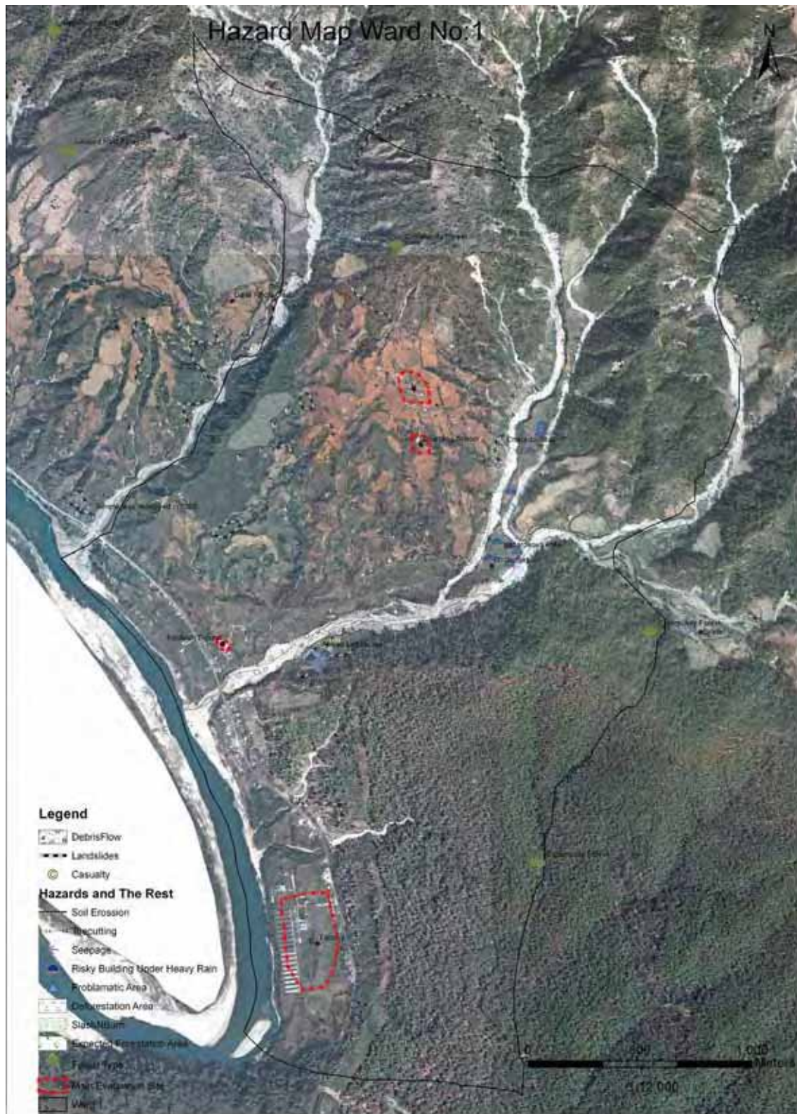
Figure 4.1.9(a) Disaster Information on Satellite Image at Step 1 of Hazard Mapping
